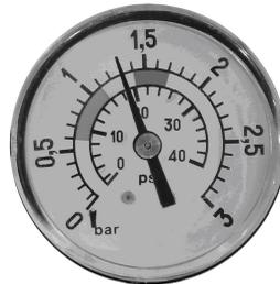
**1.3 kg/cm<sup>2</sup> - 18.5 PSI:** This pressure indicates that it is necessary to "BACKWASH"
